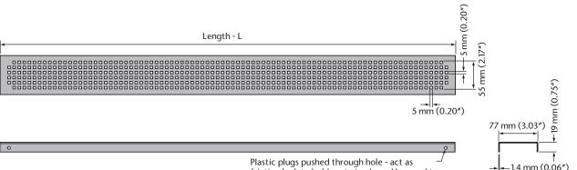
friction lock to hold grate in place. Also used to hold optional light units in position.
