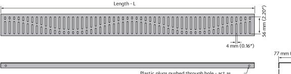
Plastic plugs pushed through hole - act as friction lock to hold grate in place. Also used to hold optional light units in position.
