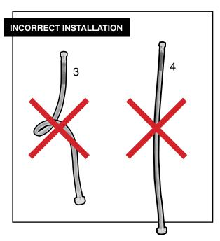
In illustration 3, the FLEX is kinked causing poor water flow.
