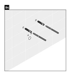
Please note if the sink will be mounted on a concrete wall application, anchors must be used.
