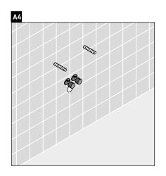
Install shut off valves according to manufacturer's installation instructions.
