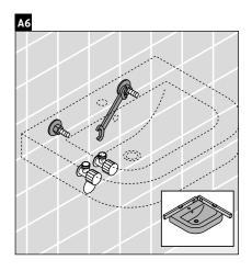
Leveling the sink: the white plastic sleeves protect the china from the metal bolt and allow for slight adjustment in the height of the sink to level it.
