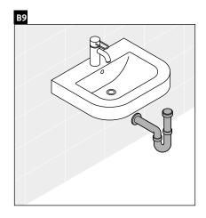
Install the p-trap according to the corresponding installation instructions.
