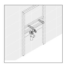
When mounting the sink on a pre-wall carrier, install the mounting bolts to the element.
