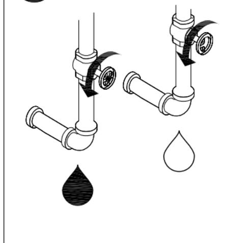
Purge the water supply system for around 30 seconds.
