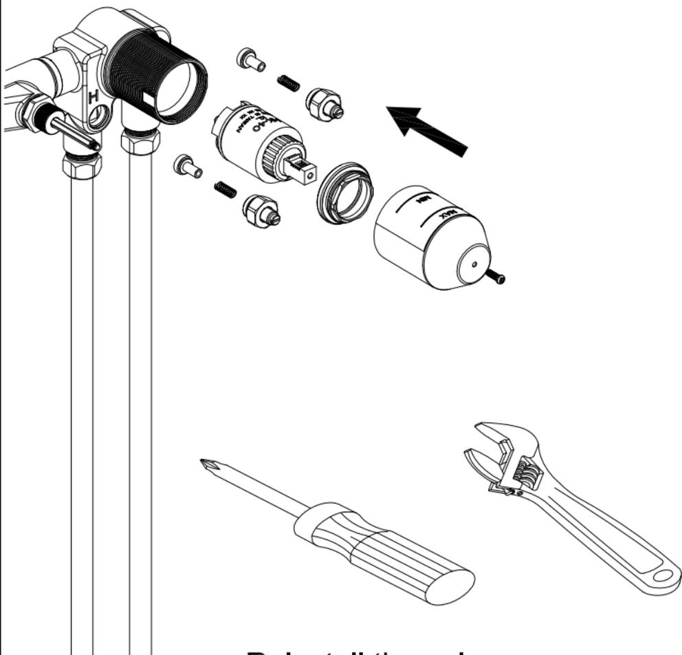
Reinstall the valve components into their original positions.
