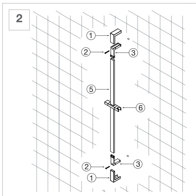
Assemble the slider (6) to the tube (5), and adjust the slider to a suitable position. Assemble the wall brackets (3) to the upper part and lower part of tube, then fix them with self-tapping screws (2), as in Fig. 2 and place the wall bracket covers (1) to the wall brackets.
