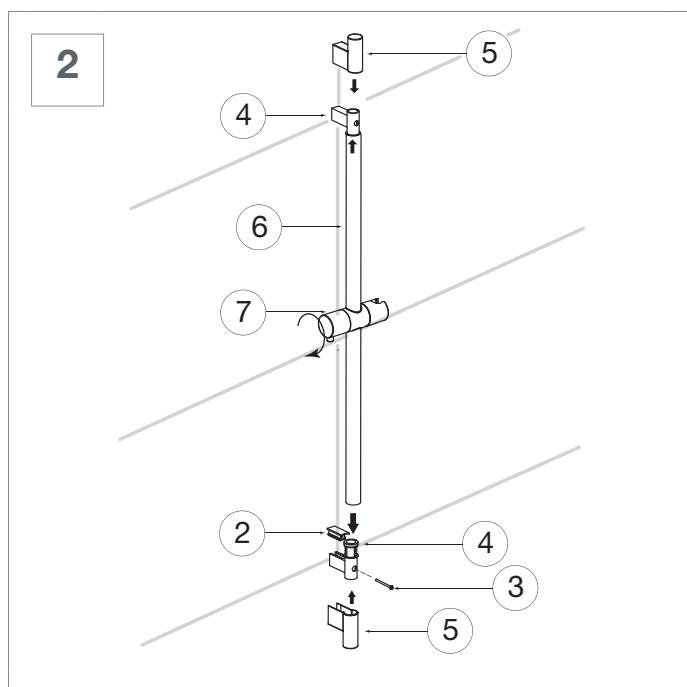
Before inserting the rail into the wall supports, slide handshower holder (7) onto the rail by turning the button on holder as shown. This handshower holder can be used either on the right or left side of the rail (Fig.2).
