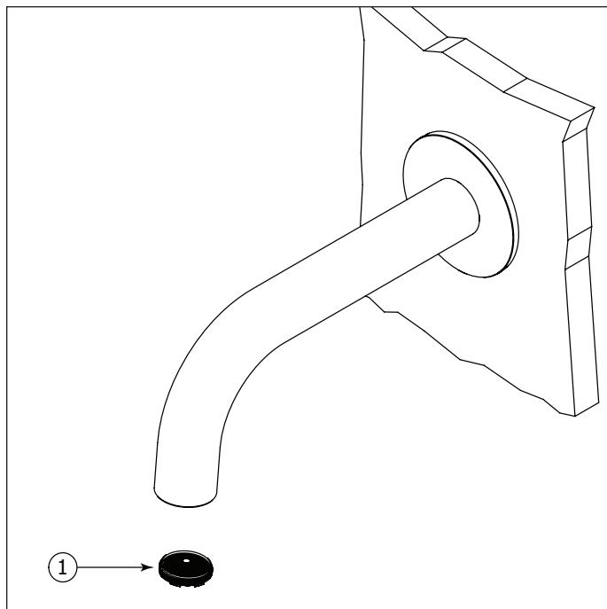
To clean the aerator (1), unscrew the aerator case from the spout. Then, pull out the aerator and soak it in a vinegar and water solution to remove lime build-up. Once parts have been cleaned, reassemble by reversing steps.
