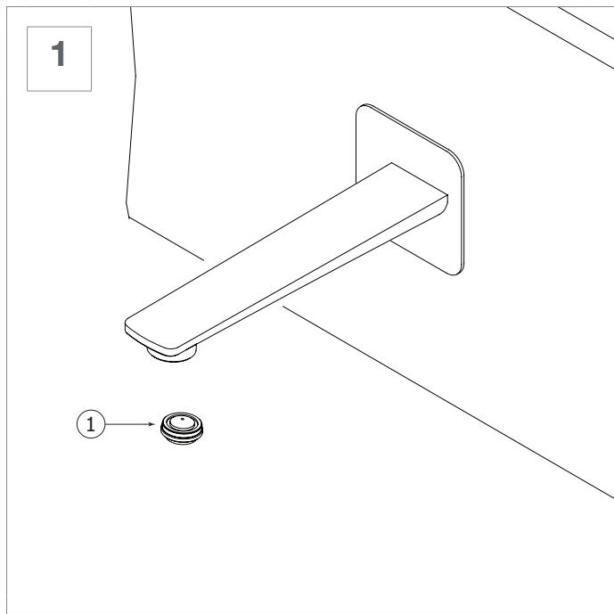
To clean the aerator (1), remove it from the spout. Then soak it in vinegar and water solution to remove lime build-up. Once parts have been cleaned, reassemble by reversing steps.
