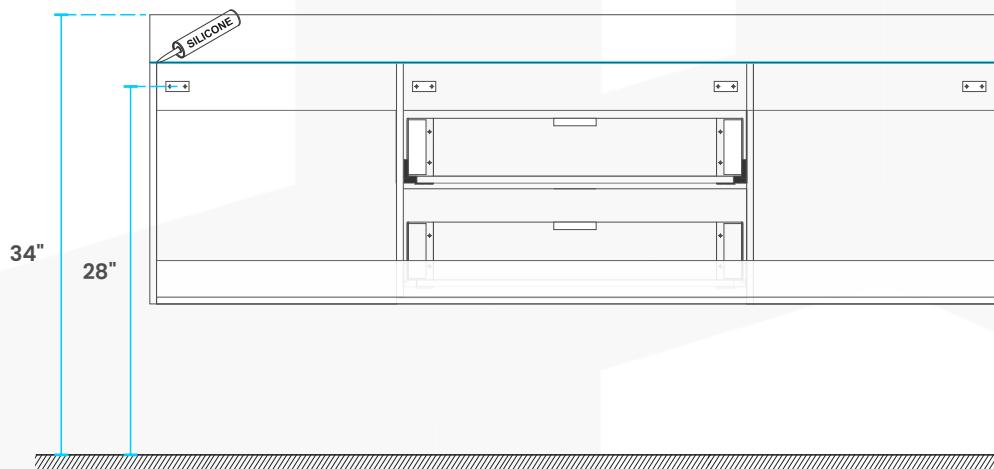
1. Align and level mounting Brackets according to horizontally reinforcement lumber and desired cabinet height.
