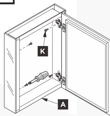
Secure mirrored side panels with provided screws (**K**) using screwdriver.
