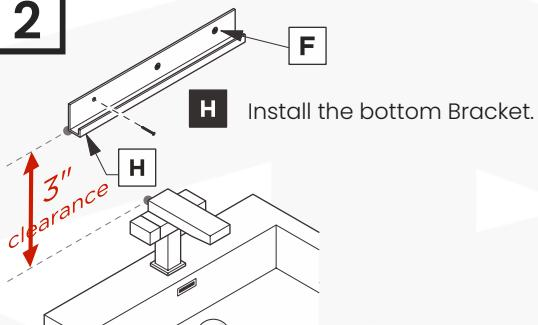
Consult an expert for the proper screw/bolts to use when attaching to various wall constructions.
