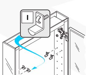
Push and twist the snap-in pins (**I**) into the place.
