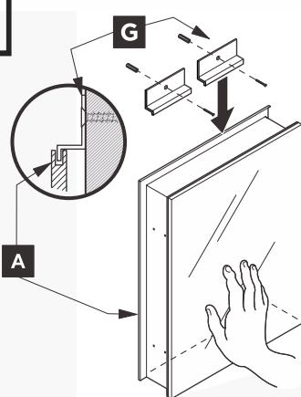
Hold the Cabinet then fit the top bracket (**G**) on the top of the cabinet then attach the bracket to the wall
